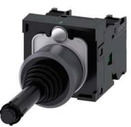
Coordinate switch, 22 mm, round, plastic with metal front ring, black, 2 switch positions, vertical, momentary contact type, with mechanical interlocking in O position, with holder, 1 NO, 1 NO, screw terminal, with laser labeling, lower case
