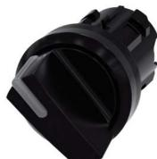
Illuminable selector switch, 22 mm, round, plastic, black, Selector switch short, 2 switch positions O<I, momentary contact type, Actuating angle 45°, 10:30h/12h
