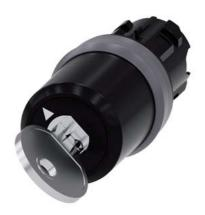
key-operated switch Siemens, 22 mm, round, plastic with metal front ring, lock number SSG10, with 2 keys, 2 switch positions O-I, latching, actuating angle 90°, 10:30h/13:30h, key removal O, with laser labeling, upper case and lower case, always upper case at the beginning of the word
