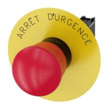
EMERGENCY STOP mushroom pushbutton, 22 mm, round, plastic, red, 40 mm, positive latching, acc. to EN ISO 13850, rotate-to-unlatch, with yellow backing plate, inscription: Arrêt d'urgence, with holder, 1 NC, screw terminal, Z=20-unit packaging
