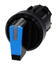
Selector switch, illuminable, 22 mm, round, plastic, blue, selector switch, short, 3 switch positions I-O<II, left latching, right momentary contact type, actuating angle 2x45°, 10:30h/12h/13:30h, with laser labeling, inscription or symbol Customerspecific selection with SIRIUS ACT configurator (CIN)
