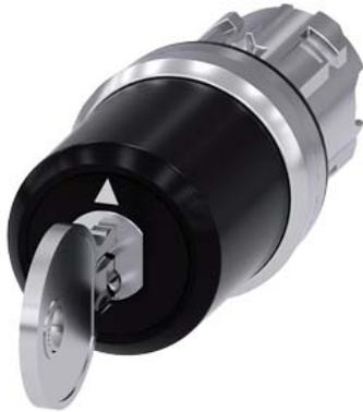
Key-operated switch BKS, 22 mm, round, metal, shiny, special lock, with 2 keys, 3 switch positions I-O<II, latching on the left, momentary contact type on the right, actuating angle 2x45°, 10:30h/12h/13:30h, key removal O+I, Note: BKS locking systems E1 - E25 supplied without key
