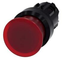
Illuminated mushroom pushbutton, 22 mm, round, plastic, red, 30 mm, momentary contact type, with laser labeling, symbol number according to, ISO 7000 or IEC 60417
