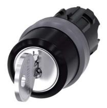
RONIS key-operated switch, 22 mm, round, plastic with metal front ring, special lock, with 2 keys, 3 switch positions I-O-II, latching, actuating angle 2x45°, 10:30h/12h/13:30h, Key removal I+II, possible special locks: SB31, 421, 455
