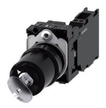
key-operated switch Siemens, 22 mm, round, plastic, lock number SSG10, with 2 keys, 2 switch positions O-I, latching, 10:30h/13:30h, key removal O+I, with holder, 1 NO+1 NC, spring-loaded terminal, with laser labeling, upper case
