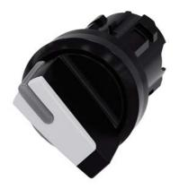
Selector switch, illuminable, 22 mm, round, plastic, white, selector switch, short, 2 switch positions O-I, latching, actuating angle 90°, 10:30h/13:30h, with laser labeling, upper case
