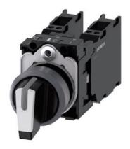
Selector switch, illuminable, 22 mm, round, plastic with metal front ring, white, selector switch, short, 3 switch positions I-O-II, latching, actuating angle 2x45°, 10:30h/12h/13:30h, with holder, 1 NO+1 NC, 1 NO+1 NC, Spring-type terminal
