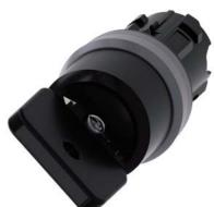
Key-operated switch O.M.R, 22 mm, round, plastic with metal front ring, lock number 73034, black, with 2 keys, 2 switch positions O-I, latching, actuating angle 90°, 10:30h/13:30h, key removal O+I, with laser labeling, lower case
