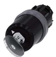
Key-operated switch BKS, 22 mm, round, plastic with metal front ring, Lock number E1 (VW), without key, 2 switch positions O-I, latching, actuating angle 90°, 10:30h/13:30h, key removal O+I, with laser labeling, upper case and lower case, always upper case at beginning of line
