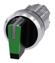
Selector switch, illuminable, 22 mm, round, metal, shiny, green, selector switch, short, 3 switch positions I>O<II, momentary contact type, actuating angle 2x45°, 10:30h/12h/13:30h
