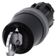
Key-operated switch IKON, 22 mm, round, plastic with metal front ring, lock number 360012K1, with 2 keys, 3 switch positions I>O<II, momentary contact type, actuating angle 2x45°, 10:30h/12h/13:30h, key removal O, with laser labeling, upper case and lower case, always upper case at beginning of line
