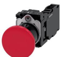
Mushroom pushbutton, 22 mm, round, plastic, red, 40mm, latching, pull-to-unlatch mechanism, with holder, 1 NO+1 NC, screw terminal, with laser labeling, inscription or symbol Customer-specific selection with SIRIUS ACT configurator (CIN)
