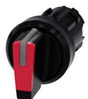
Selector switch, illuminable, 22 mm, round, plastic, red, selector switch, short, 3 switch positions I>O<II, momentary contact type, actuating angle 2x45°, 10:30h/12h/13:30h, with laser labeling, upper case
