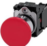
Mushroom pushbutton, 22 mm, round, metal, shiny, red, 40mm, latching, pull-tounlatch mechanism, with holder, 1 NC, screw terminal, Z=20-unit packaging
