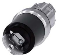
Key-operated switch IKON, 22 mm, round, metal, shiny, lock number 360012K1, with 2 keys, 2 switch positions O-I, latching, actuating angle  $90^{\circ}$ , 10:30h/13:30h, Key removal O+I
