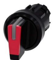
Selector switch, illuminable, 22 mm, round, plastic, red, selector switch, short, 3 switch positions I>O<II, momentary contact type, actuating angle  $2x45^{\circ}$ , 10:30h/12h/13:30h
