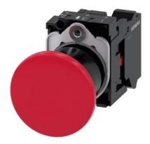
Mushroom pushbutton, 22 mm, round, plastic, red, 40mm, latching, pull-to-unlatch mechanism, with holder, 1 NC, spring-type terminal, with laser labeling, inscription or symbol Customer-specific selection with SIRIUS ACT configurator (CIN)
