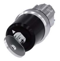
key-operated switch Siemens, 22 mm, round, metal, shiny, lock number SSG10, with 2 keys, 2 switch positions O-I, latching, actuating angle  $90^\circ$ , 10:30h/13:30h, key removal O+I
