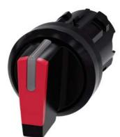
Selector switch, illuminable, 22 mm, round, plastic, red, selector switch, short, 3 switch positions I-O-II, latching, actuating angle  $2x45^{\circ}$ , 10:30h/12h/13:30h, with laser labeling, upper case
