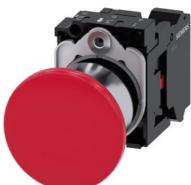
Mushroom pushbutton, 22 mm, round, metal, shiny, red, 40mm, latching, pull-tounlatch mechanism, with holder, 1 NC, spring-type terminal, with laser labeling, upper case
