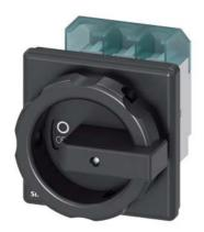
SENTRON, Switch disconnector 3LD, main switch, 3-pole, lu: 63 A, Operating power / at AC-23 A at 400 V: 22 kW, front-mounted, rotary operating mechanism, black, 4-hole mounting of the handle
