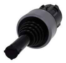
Coordinate switch, 22 mm, round, plastic with metal front ring, black, 4 switch positions, latching, without mechanical interlocking, Z=50-unit packaging
