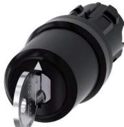
Key-operated switch IKON, 22 mm, round, plastic, lock number 360012K1, with 2 keys, 3 switch positions I-O<II, left latching, right momentary contact type, actuating angle 2x45°, 10:30h/12h/13:30h, key removal O+I, with laser labeling, upper case and lower case, always upper case at beginning of line
