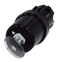
Key-operated switch BKS, 22 mm, round, plastic, Lock No. E2 (VW), without key, 2 switch positions O-I, latching, actuating angle  $90^\circ$ , 10:30h/13:30h, key removal O+I, with laser labeling, upper case and lower case, always upper case at beginning of line
