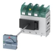
SENTRON, Molded case switch 3LD5 UL, Main switch, 4-pole, certified according to UL489 UL60947-4-1 and IEC60947-3, UL: 125A, SCCR 65kA at 480VAC, Operating power at 480VAC 3-phase: 75hp, IEC: 125A, Operating power at AC-23A at 400V: 55kW, floor mounting with door coupling rotary operating mechanism, defeatable, Standard, 4-hole mounting of the handle, without tolerance compensation, incl. terminal covers for the infeed side
