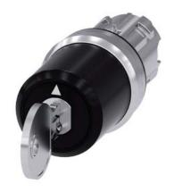
Key-operated switch BKS, 22 mm, round, metal, shiny, lock number S1, with 2 keys, 3 switch positions I>O<II, momentary contact on the left, latching on the right, actuating angle 2x45°, 10:30h/12h/13:30h, key removal O, with laser labeling, lower case
