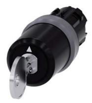
key-operated switch Siemens, 22 mm, round, plastic with metal front ring, lock number SSG10, with 2 keys, 3 switch positions I>O<II, momentary contact on the left, latching on the right, actuating angle 2x45°, 10:30h/12h/13:30h, key removal O+II, with laser labeling, upper case
