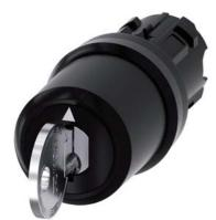
Key-operated switch IKON, 22 mm, round, plastic, special lock, with 2 keys, 3 switch positions I-O-II, latching, actuating angle 2x45°, 10:30h/12h/13:30h, Key removal I+O+II
