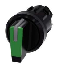
Selector switch, illuminable, 22 mm, round, plastic, green, selector switch, short, 3 switch positions I-O<II, left latching, right momentary contact type, actuating angle  $2x45^{\circ}$ , 10:30h/12h/13:30h, with laser labeling, upper case and lower case, always upper case at the beginning of the word
