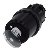
Key-operated switch BKS, 22 mm, round, plastic, lock number S1, with 2 keys, 2 switch positions O-I, latching, actuating angle  $90^{\circ}$ , 10:30h/13:30h, key removal I, with laser labeling, upper case
