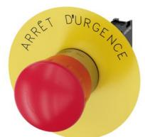
EMERGENCY STOP mushroom pushbutton, 22 mm, round, metal, shiny, red, 40 mm, positive latching, acc. to EN ISO 13850, rotate-to-unlatch, with yellow backing plate, inscription: Arrêt d'urgence, with holder, 1 NC, screw terminal
