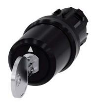
Key-operated switch BKS, 22 mm, round, plastic, lock number S1, with 2 keys, 3 switch positions I-O-II, latching, actuating angle  $2x45^\circ$ , 10:30h/12h/13:30h, key removal I, with laser labeling, upper case and lower case, always upper case at beginning of line
