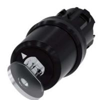
Key-operated switch BKS, 22 mm, round, plastic, Lock number E1 (VW), without key, 2 switch positions O-I, latching, actuating angle 90°, 10:30h/13:30h, key removal O, with laser labeling, upper case and lower case, always upper case at the beginning of the word
