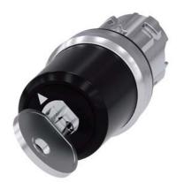
key-operated switch Siemens, 22 mm, round, metal, shiny, lock no. STGH10, with 2 keys, 2 switch positions O-I, latching, actuating angle  $90^\circ,\,10:30h/13:30h,$  key removal O+I, with laser labeling, lower case
