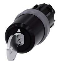
key-operated switch Siemens, 22 mm, round, plastic with metal front ring, lock number SSG10, with 2 keys, 3 switch positions I>O<II, momentary contact type, actuating angle 2x45°, 10:30h/12h/13:30h, key removal O, with laser labeling, inscription or symbol customer-specific selection with SIRIUS ACT configurator (CIN)
