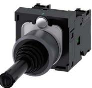
Coordinate switch, 22 mm, round, plastic with metal front ring, black, 2 switch positions, horizontal momentary contact type, without mechanical interlocking, in O position, with holder, 1 NO, 1 NO, screw terminal, with laser labeling, upper case and lower case, always upper case at beginning of line
