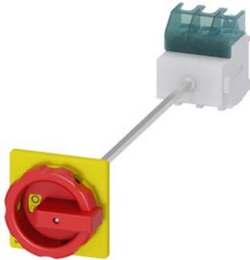
SENTRON, Switch disconnecter 3LD, emergency switching-off switch, 3- pole, Iu: 63 A, operating power / at AC-23 A 400 V: 22 kW, floor mounting with door coupling, rotary operating mechanism, Red / yellow, 4-hole mounting of the handle
