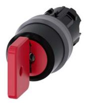
Key-operated switch O.M.R, 22 mm, round, plastic with metal front ring, lock number 73037, red, with 2 keys, 3 switch positions I>O<II, momentary contact type, actuating angle  $2x45^{\circ}$ , 10:30h/12h/13:30h, key removal O, with laser labeling, upper case and lower case, always upper case at the beginning of the word
