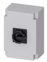
SENTRON, Switch disconnector 3LD, main switch, 3-pole, lu: 125 A, Operating power / at AC-23 A at 400 V: 45 kW, molded-plastic encapsulation for inch cable gland, 1 NC, 1 NO, rotary operating mechanism, black
