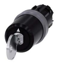
key-operated switch Siemens, 22 mm, round, plastic with metal front ring, lock number SSG10, with 2 keys, 3 switch positions I-O<II, left latching, momentary contact type on the right, actuating angle  $2x45^\circ$ , 10:30h/12h/13:30h, key removal O, with laser labeling, upper case and lower case, always upper case at the beginning of the word
