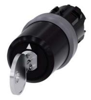
key-operated switch Siemens, 22 mm, round, plastic with metal front ring, lock number SSG10, with 2 keys, 3 switch positions I-O<II, left latching, momentary contact type on the right, actuating angle  $2x45^{\circ}$ , 10:30h/12h/13:30h, key removal O, with laser labeling, upper case
