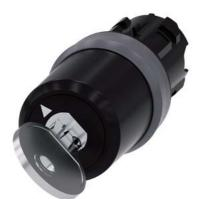
Key-operated switch BKS, 22 mm, round, plastic with metal front ring, Lock No. E7 (VW), without key, 2 switch positions O-I, latching, actuating angle 90°, 10:30h/13:30h, key removal O, with laser labeling, inscription or symbol Customer-specific selection with SIRIUS ACT configurator (CIN)
