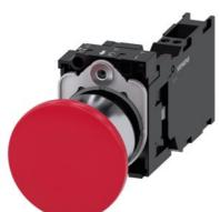
Mushroom pushbutton, 22 mm, round, metal, shiny, red, 40mm, latching, pull-tounlatch mechanism, with holder, 1 NO+1 NC, spring-type terminal, with laser labeling, symbol number according to, ISO 7000 or IEC 60417
