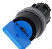
Key-operated switch O.M.R, 22 mm, round, plastic with metal front ring, lock number 73038, blue, with 2 keys, 2 switch positions O-I, latching, actuating angle 90°, 10:30h/13:30h, key removal O+I, with laser labeling, inscription or symbol Customer-specific selection with SIRIUS ACT configurator (CIN)
