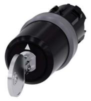
Key-operated switch BKS, 22 mm, round, plastic with metal front ring, lock number S1, with 2 keys, 3 switch positions I>O<II, momentary contact type, actuating angle 2x45°, 10:30h/12h/13:30h, key removal O, Z=50-unit packaging
