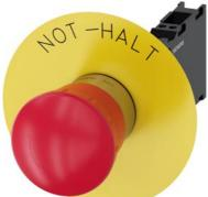
EMERGENCY STOP mushroom-type actuator, 22 mm, round, metal, shiny, red, 40 mm, positive latching, according to EN ISO 13850, rotate-to-unlatch, with yellow backing plate, inscription: NOT-HALT, with holder, 1 NO+1 NC, spring-type terminal, Z=20-unit packaging
